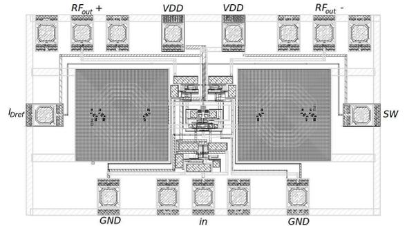
Figure 8: Layout of the LNA
