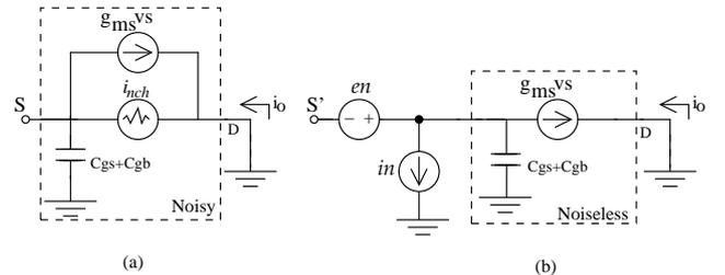
Figure 2: Two port small signal representation. (a) Transistor as a noisy element, (b) transistor as a noiseless element
