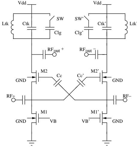
Figure 3: LNA's schematic
