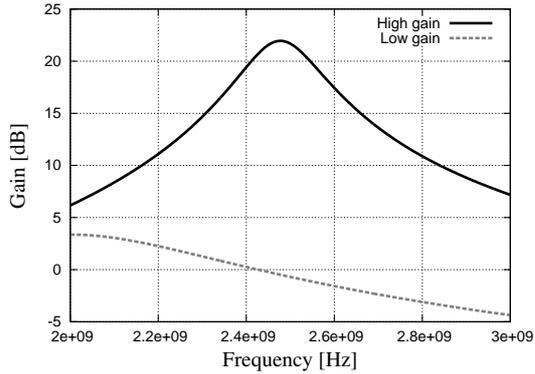
Figure 5: Simulated voltage gain of the LNA
