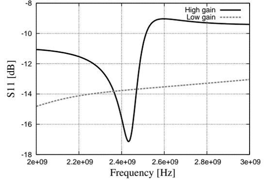
Figure 7: Simulated return loss of the LNA
