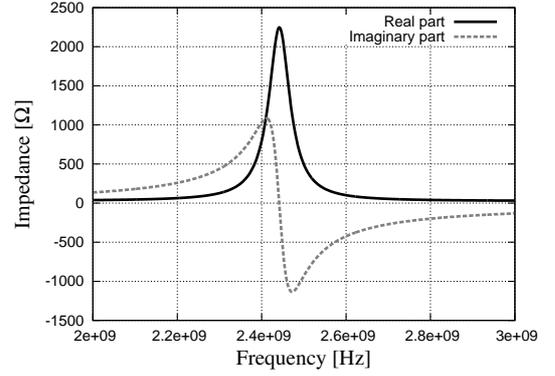
Figure 4: Simulated input impedance of the Sigma-Delta converter
