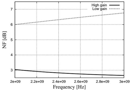
Figure 6: Simulated noise figure of the LNA
