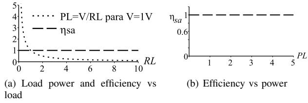
Fig. 5. PETO for lossless source
