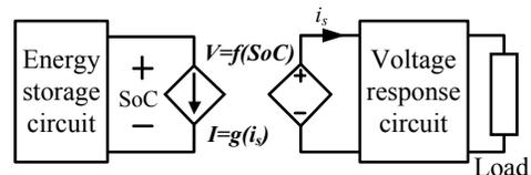
Fig. 1. Combined electrical-circuit based model.
