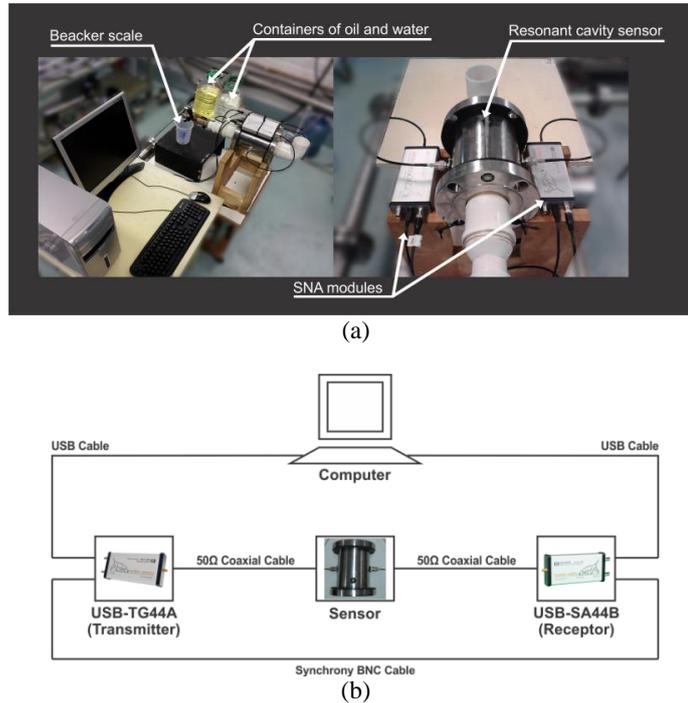
Figure 2. Details of the experimental set-up (a) and a block diagram of the implemented set-up (b).
