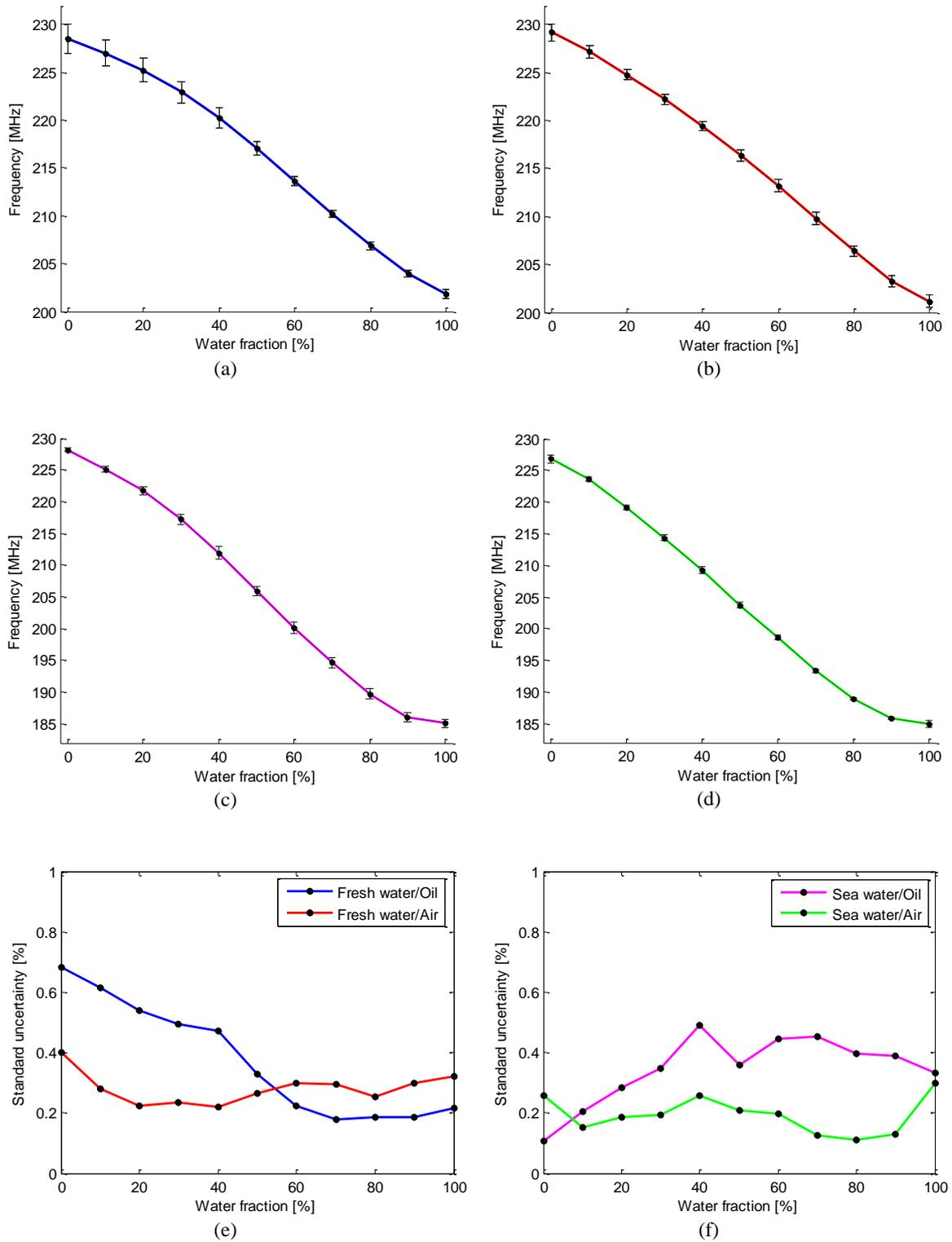
Figure 3. Standard deviation from the average values of the frequency of first resonant mode for fresh water/oil (a), fresh water/air (b), sea water/oil (c), and sea water/air (d) mixtures. Percentage of standard uncertainty for the fresh water (e) and sea water (f) mixtures.
