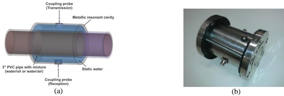
Figure 1. Sketch (a) and photograph (b) of the resonant cavity sensor.
