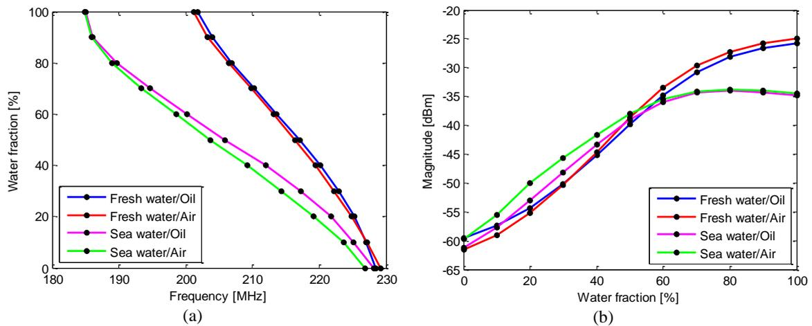
Figure 4. A comparison between all curves of the water fraction as function of resonant frequency (a) and signal magnitude as function of water fraction (b).
